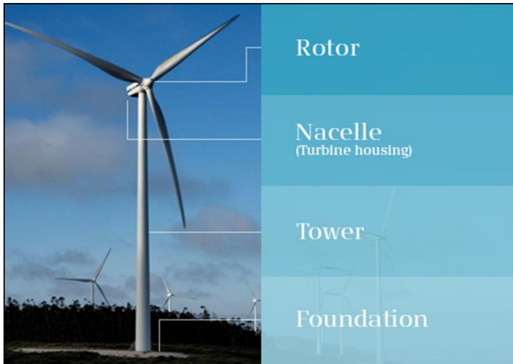
Plate 4-1 Wind turbine components
